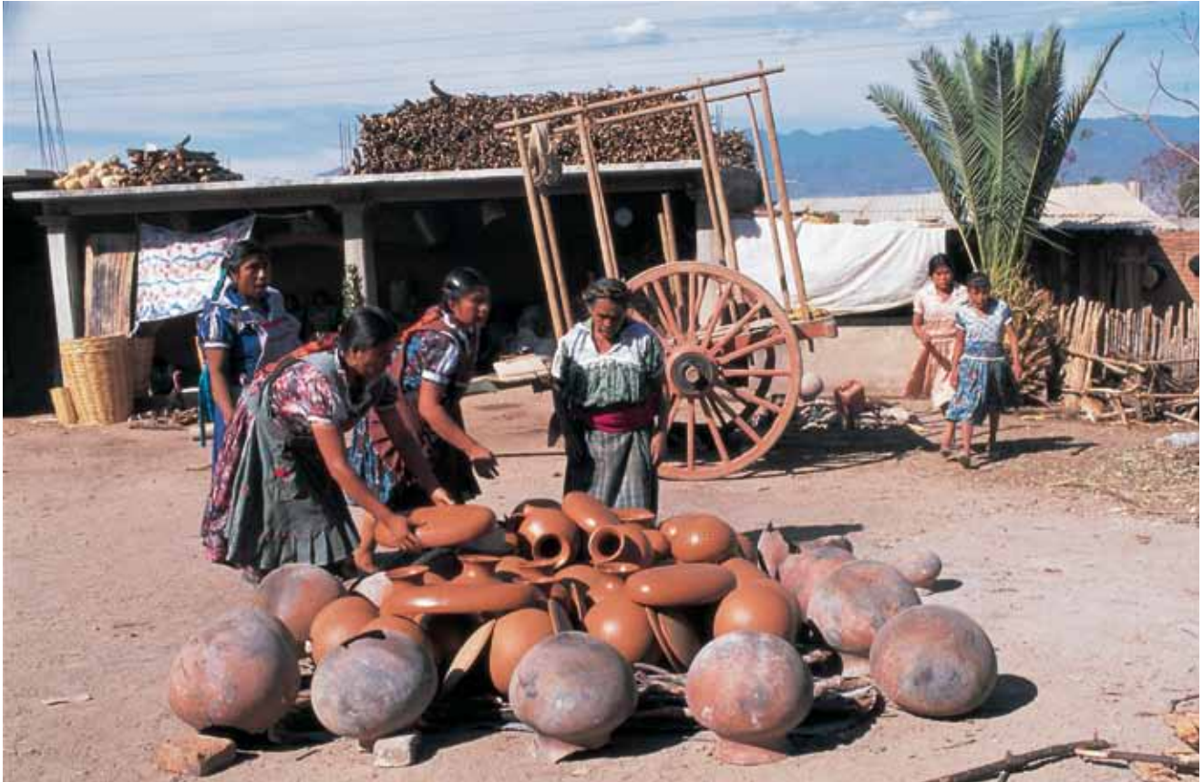
East Valley Zapotec potters tumblestack pots for a bonfiring; already fired pots and shards are used to insulate the stack.
