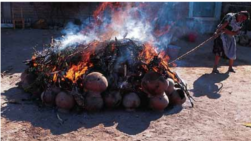
As the wood settles during the firing, it is repositioned with a long agave stalk to prevent cold spots.
