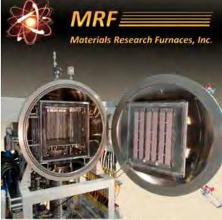
2000°C 1ft<sup>+</sup> Furnace with oil-free Turbo Pumping system
